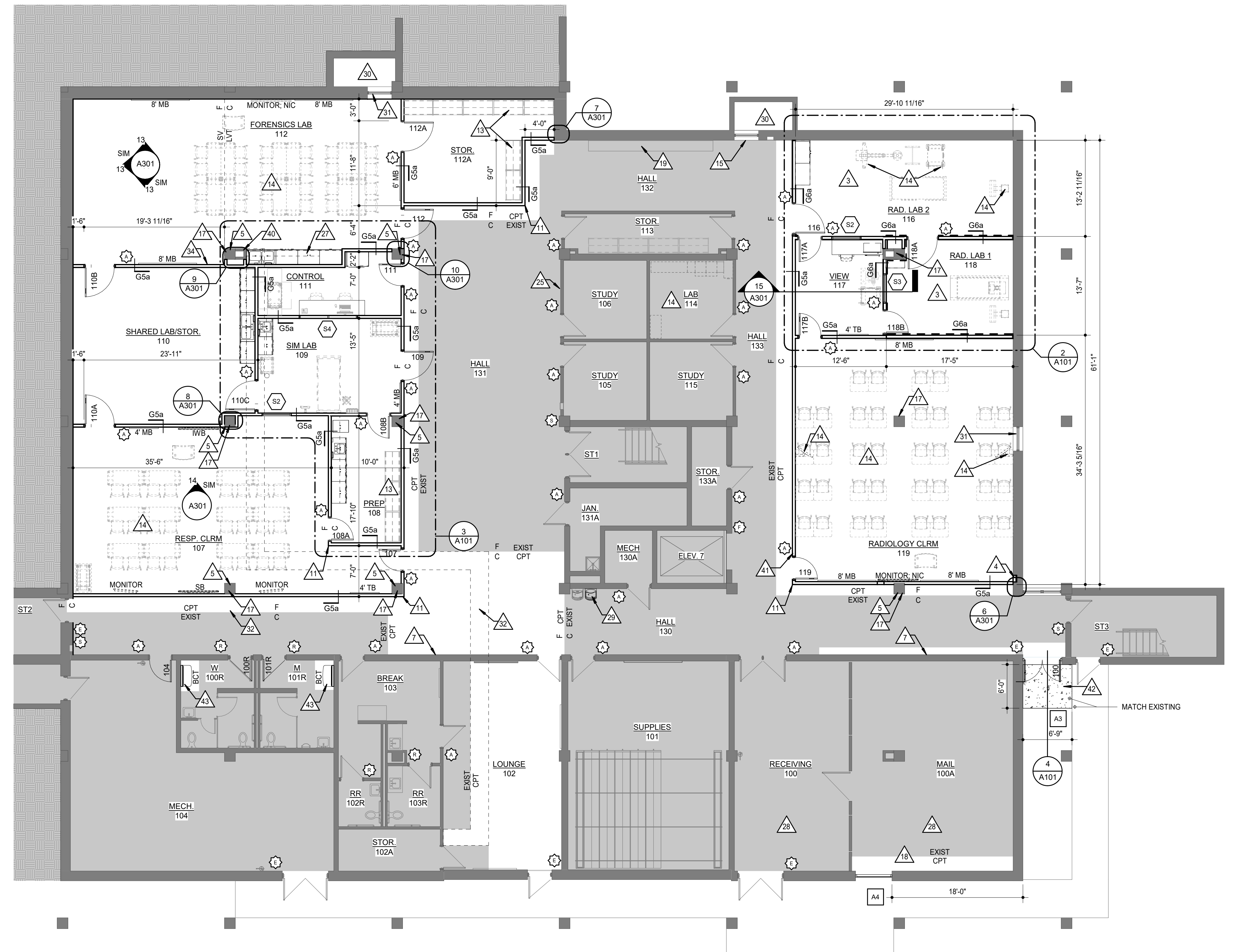
1 ARCHITECTURAL FLOOR PLAN - LOWER LEVEL 1/8" = 1'-0"
